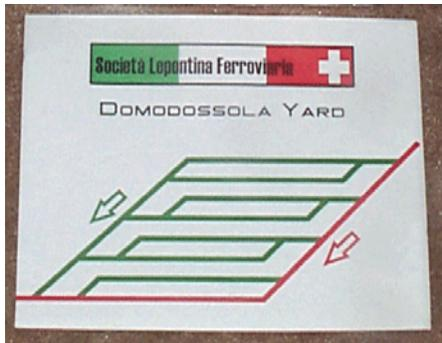
The next step is to draw some sort of track diagram to mount in the frame. I did mine on the computer using a basic drawing program and printed it on a color inkjet printer. You could also do it freehand using any combination of colored markers, colored tape, and dry transfer lettering. When laying out your artwork, consider where you will need to drill holes to mount toggle switches and other controls; be sure to leave enough back side room between the components and at the edges!
