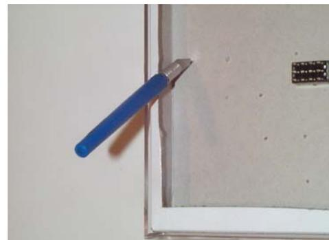
the control panel and temporarily install switches in them. You can then cut the remaining holes without things shifting.
