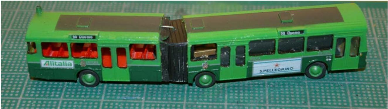
To camouflage the unsightly gap around the semi-cylindrical 'diaphragm' I installed strips of thin rubber to the rear portion of the bus. In the photo above, all of the windows are not yet installed - very tricky at the articulation joint because there's little space left.
