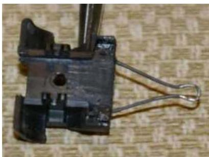
Drill two holes in the dolly, insert the ends, line everything up, and glue the wire in place with CA.
