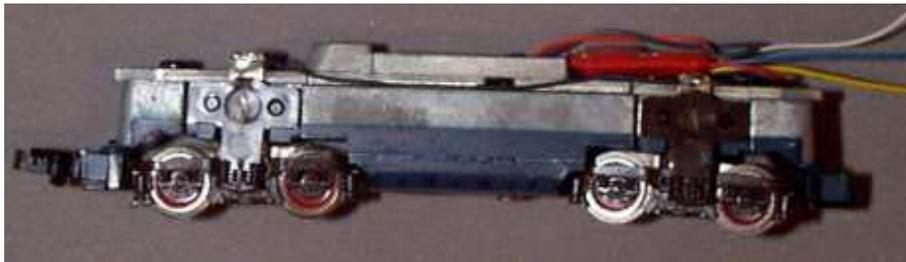
**Figure 3: Location of the decoder atop the mechanism**
