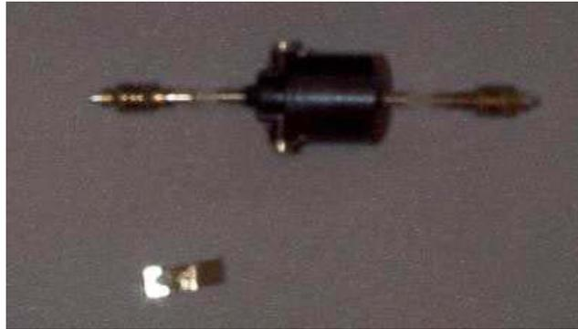
**Figure 1: Motor with underside contact removed**
